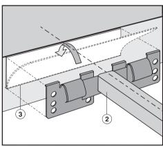
■ Position and attach the spring clips
